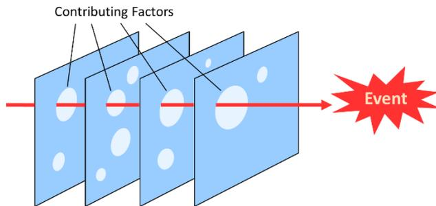
In safety-critical systems, safety is created by setting up staggered safety barriers. In the figure, this is illustrated in accordance with J. Reason's "Swiss Cheese Model".
